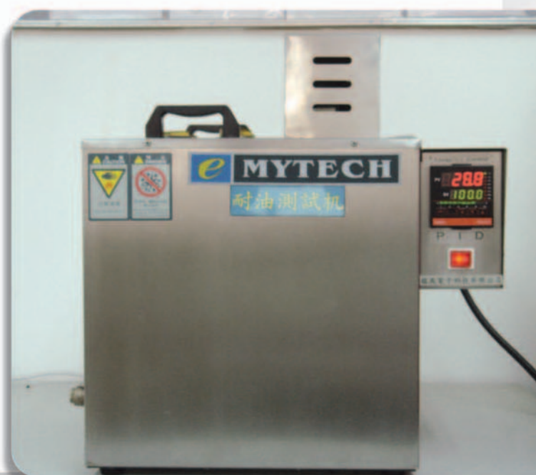
Oil Resistance Test 耐油測試
