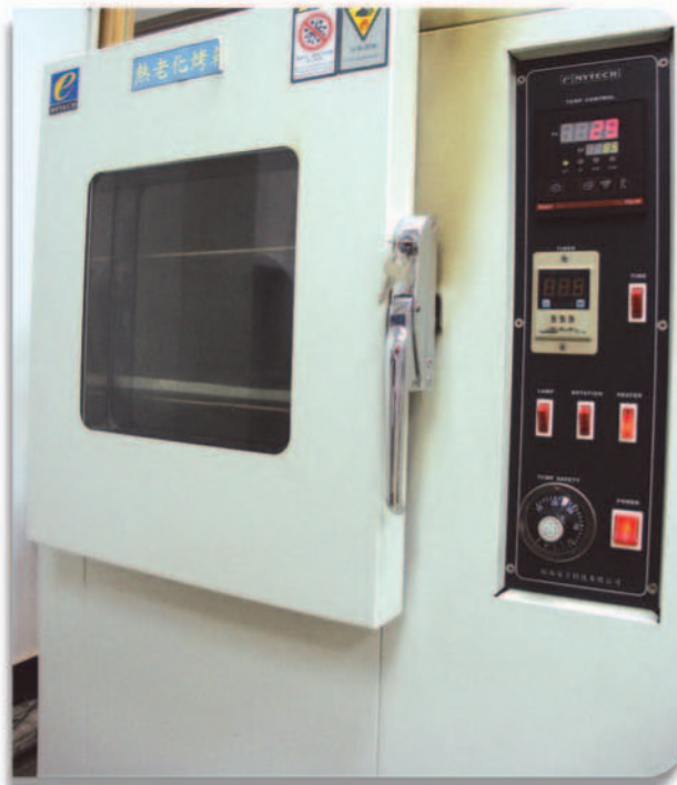
Constant Temperature Humidity Chamber 恆溫測試
